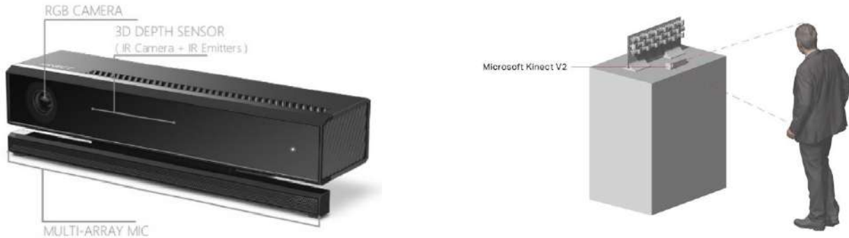
Figure 2. Left shows Microsoft Kinect V2 device (Basu, 2016) and right shows sensor's area coverage of Kinect's sensor (source: authors).
